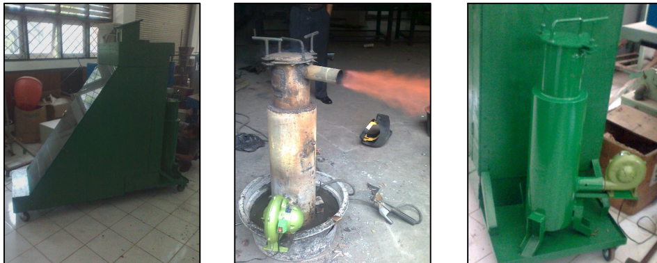
Gambar 1. Oven Pengering Tenaga Surya – Syngas ( Hybrid Solar Dryer )
