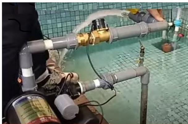
Gambar 4. Instalasi Pompa Dengan System Kontrol Pressure Dan Flow Switch
